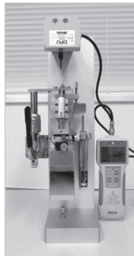
Fig.1 Device for measuring retentive force
