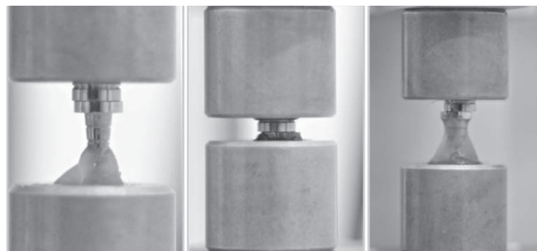
Fig.4 Possible misalignment between the magnetic attachment and the keeper
