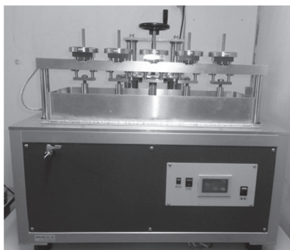
Fig. 4 Insertion/removal testing machine
