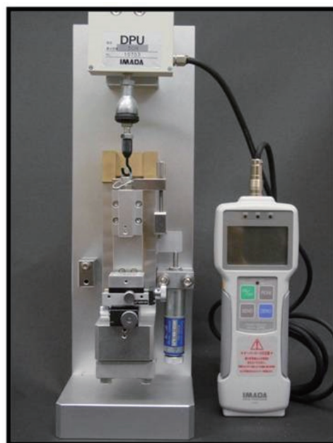
Fig. 2 Simplified attractive force measuring machine
