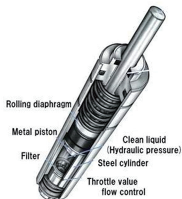
Fig4 Inner structure of dashpot
