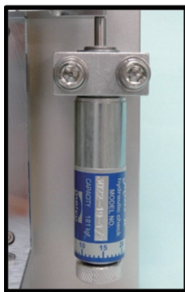
Fig.5 Dashpot (KINECHECK, meiyu)
