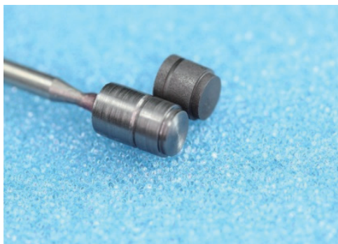
Fig.1 Trial graphite pattern made from carbon rod
