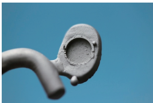
Fig.6 As-cast after heating and storing (700°C, 20 minutes)
