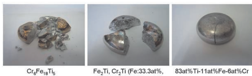
Fig.9 The alloys whose composition was almost intermetallic compounds and the side containing much titanium
