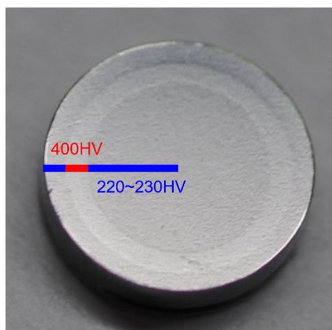
Fig. 4 Mating face view of magnetic assembly and its hardness
