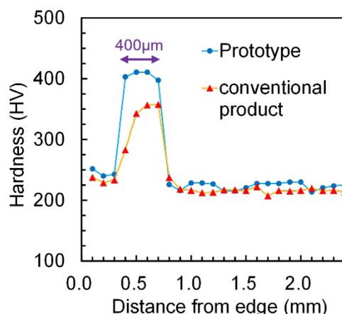
Fig. 3 Hardness profile of the mating face of magnetic assembly
