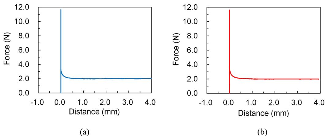
Fig. 1 Retentive force curve. (a) prototype, (b) conventional product
