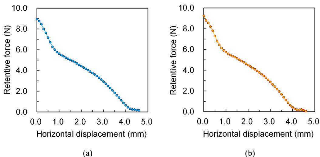
Fig.2 Retentive force against horizontal displacement (a) prototype, (b) conventional product
