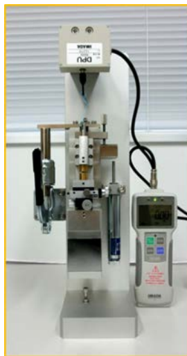
Fig. 1 Device for measuring retentive force
