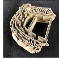
Fig.12 The support was attached on the occlusal surface of the framework.
