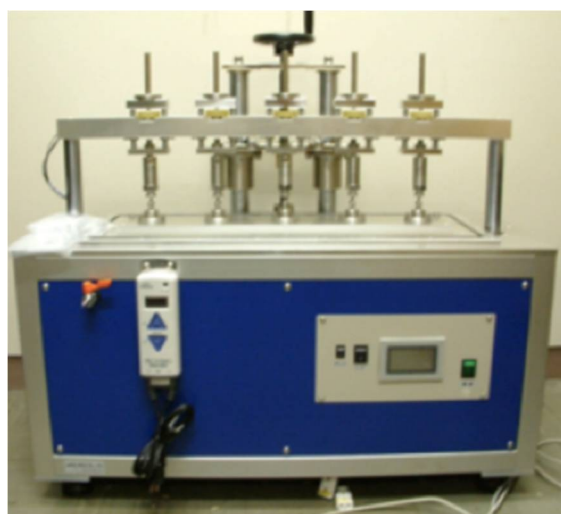
Fig. 4 Cyclic loading testing machine for tensile test
