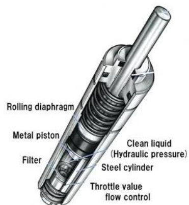
Fig4 Inner structure of dashpot
