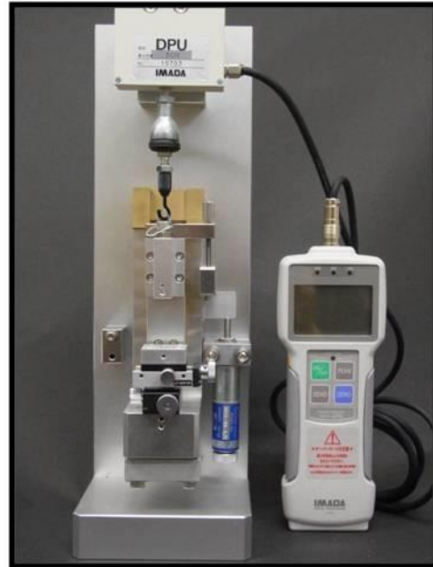
Fig. 2 Simplified attractive force measuring machine
