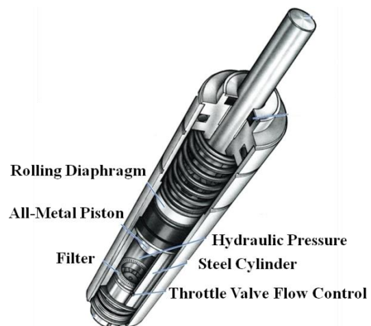
Fig.6 the inner structure of a dash-pot
