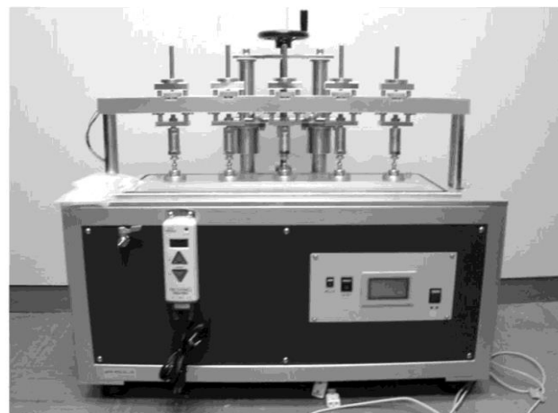
Fig. 3 Cyclic loading testing machine for tensile test
